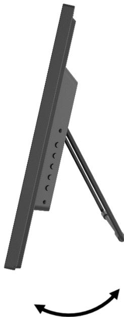
\*Forcing the stand open at the rear may cause damage. In addition, if the angle of the stand is not sufficiently inclined, it may fall over. Take care not to tip the main unit when in use.
